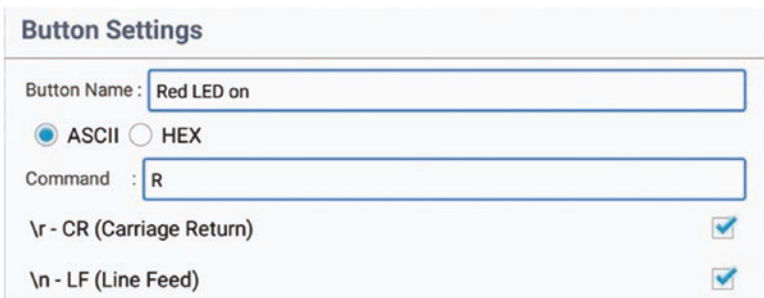
Figure 16-3. Bluetooth Terminal HC-05 button setup to control LEDs
