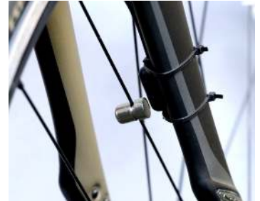
Figure 10.4 Bicycle computer sensor and magnet.
