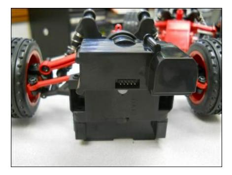
The five-pin connector that comes from the control module is shown in the following image:
