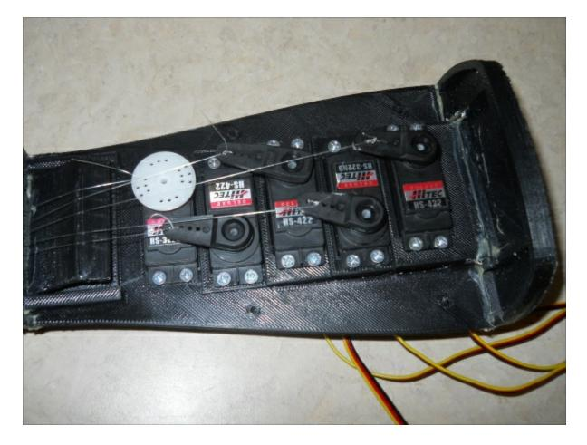
Connect each of the digits to a servo, and then connect the entire hand to a bracket; this will act as the wrist. You'll also connect this to a servo that can turn the wrist.
