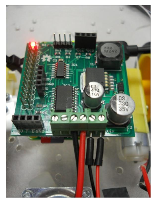
3. Then, connect the second drive connector to the motor 2
