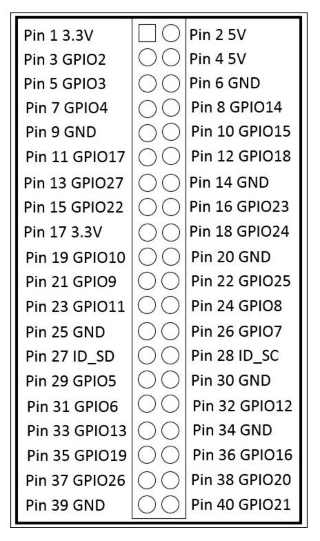
You'll need to connect to the 5 volt connection of the Raspberry Pi Zero, pin 2. You also need to connect to the GND, which is pin 6 on Raspberry Pi. Pin 16 (GPIO 23) is used as an output trigger pin and pin 18 (GPIO 24) as an input to time the echo from the sonar sensor.
