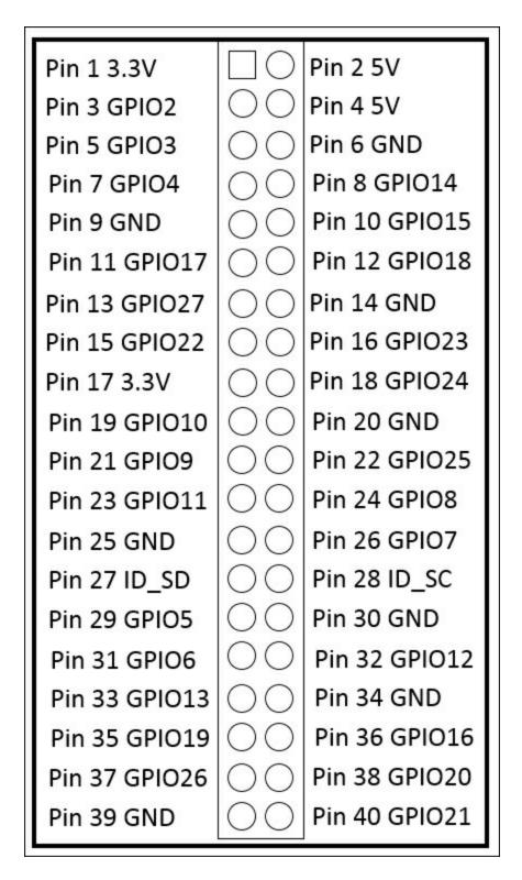
5. You'll use **Pin1 3.3V** for the 3.3-volt signal and **Pin 9 GND** for the ground signal. You'll connect one of the GPIO pins so that you can create the 320 Hz, 10 percent duty cycle signal to enable the
