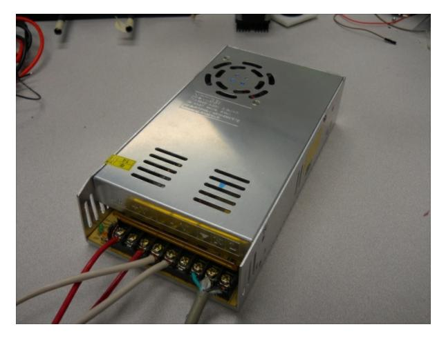
The connections on the power supply are clearly marked; you'll connect the 6-volt power supply and GND connections to the connections marked BAT on the servo controller.
