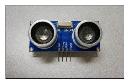
The device is an HC-SR04 and they are available at most online electronics retailers. Now let's connect the device to Raspberry Pi Zero. In order to do this, first let's look at the layout of the GPIO pins on Raspberry Pi Zero:
