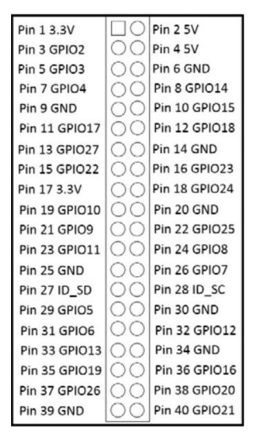
The purpose of some of these pins is very clear. Pins 1 and 17 are available to supply 3.3 volts, pins 2 and 4 supply 5 volts, and pins 9, 25, 39, 6, 14, 20, 30, and 34 are all connected to ground on Raspberry Pi Zero. The rest of the pins have various capabilities, which you'll learn in this chapter. Let's start with the pins that can be used to supply a simple DC signal to the outside world.
