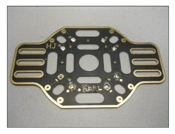
Note the + and – connections; each connection will be soldered to all the ESCs. The following is an image of the motor controller:
