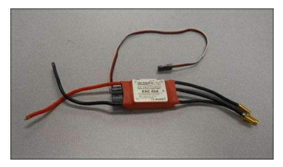
The red and black wire connectors are the connectors that are soldered to the bottom plate of the frame. The other three
