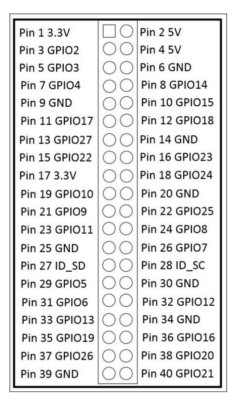
You need to connect these pins on the Raspberry Pi Zero GPIO to the pins on the H-bridge, as shown in the following table:
