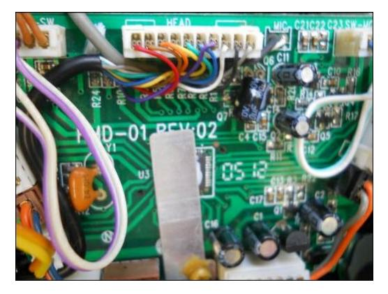
There are only two wires that you are interested in. The first is the black wire, which is the GND for the Robosapien system. The second is the white wire. This is the serial connection that controls the command for the Robosapien.
