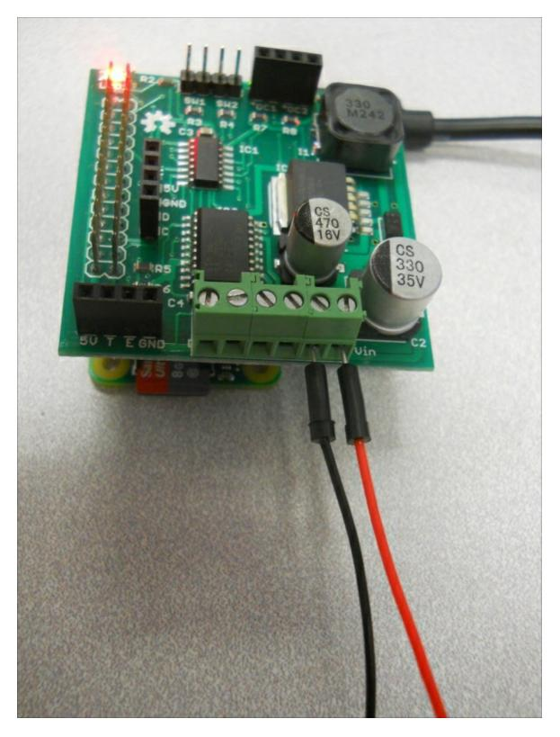
2. Next, connect one of the drive signals to the motor 1 connector on the board. Connect motor 1 to the right motor and motor 2 to the
