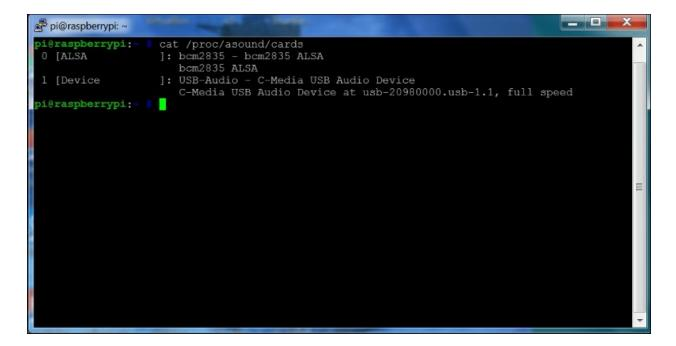
There are two possible audio devices that you can use. The first is the internal Raspberry Pi audio, which is connected to the audio port, and the second is the USB audio plugin. You could use the USB audio plugin to record the sound and the Raspberry Pi for the audio output to play the sound, though it is easier to just use the USB audio plugin to create and record sound.
