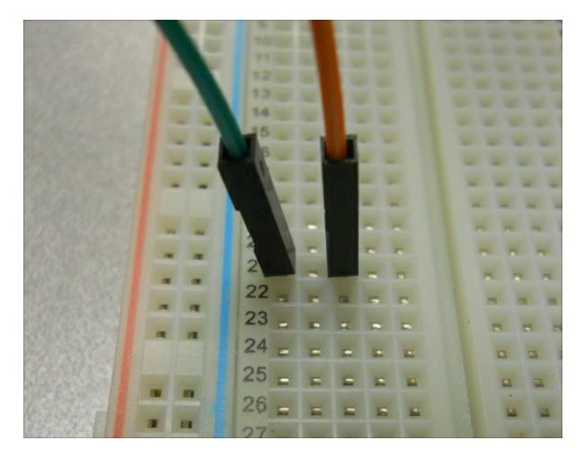
The two rows on each side of the board are generally designed to provide power, so they are connected up and down. Connect pin 2, 3 volts, to the + connection and pin 6, GND, to the + and – rows of the breadboard, as shown:
