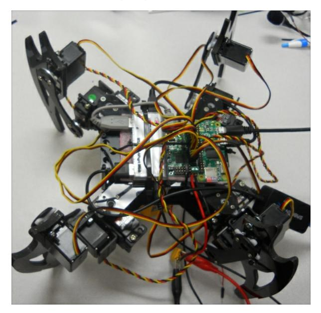
The Raspberry Pi Zero is in the middle, the motor controller is to the right, and the powered hub to the left. The alligator clips below are connected to a power supply; eventually you'll want to connect these to a battery.
