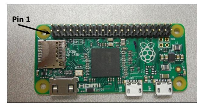
Here is a listing of the pins and their connection to the Raspberry Pi Zero:
