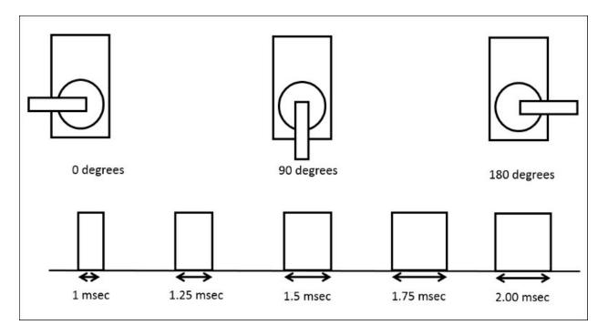
These pulses are sent out with a repetition rate of 60 Hz. You can position the servo at any angle by setting the correct control pulse.
