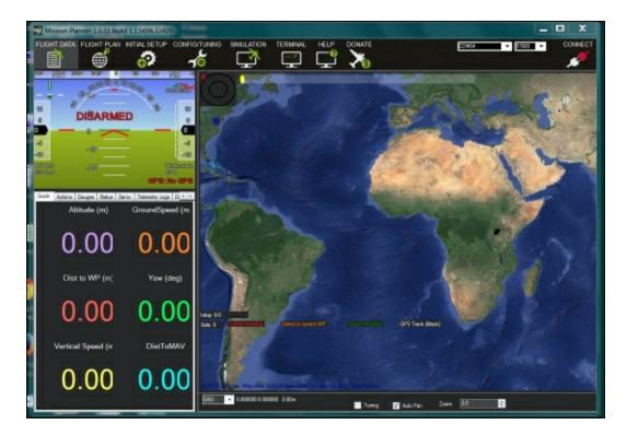
This is the basic screen. You'll then need to configure your radio's COM port and then press the **CONNECT** button in the corner on the upper right-hand side of the screen. As you move the quadcopter around, you will see the measurements change. If you are having problems connecting to the Pixhawk, there is lot of help available on
