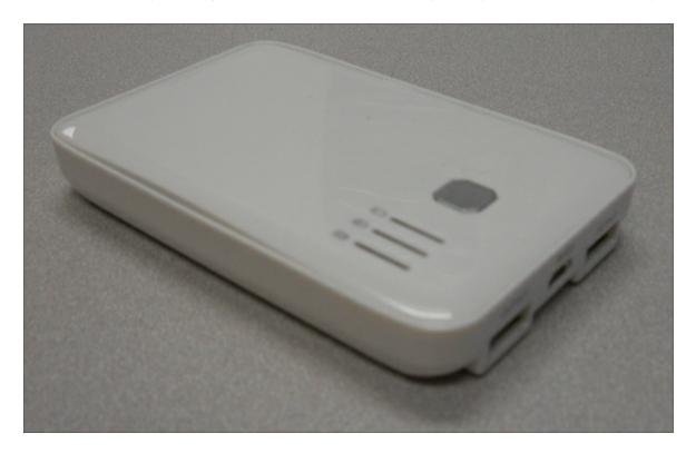
In both cases, make sure that the unit can supply enough current. You'll need a supply that can provide at least 1000 mA at 5 volts. There are two USB charge connections on this battery which makes it
