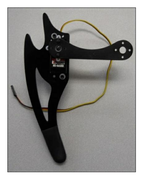
3. Complete the leg by connecting two of the servo brackets together at right angles, mounting the HS-645MG onto one of the brackets, and then connecting this servo to the interconnecting piece, as shown:
