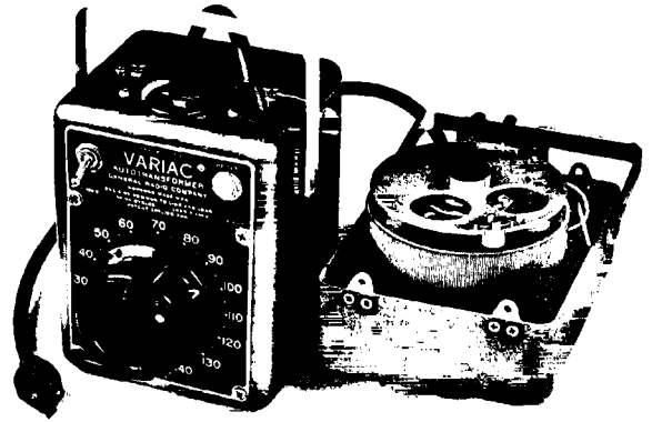
Figure 1.129. A powerline variable transformer ("Variac") lets you adjust the ac input voltage to something you are testing. Here a 5 A unit is shown, both clothed and undressed.
